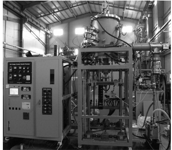
Fig. 1. Growth system of Resistant heating method for SiC single crystal using graphite heating element.
