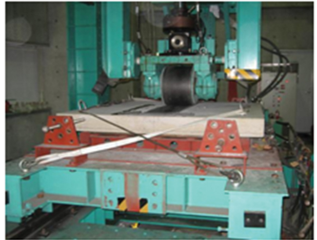
Fig. 1. Fatigue test under running wheel load equipment.
