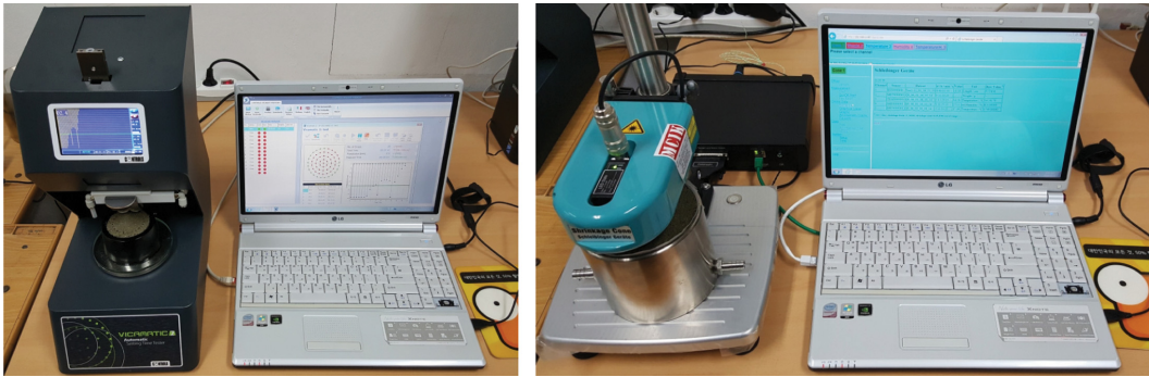
Fig. 3. Experimental apparatus for the setting-time (left) and shrinkage (right).
