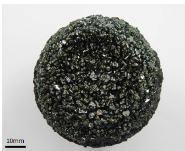
Fig. 3. A photograph of SiC crystals grown on the upper part of source materials inside of the crucible.
