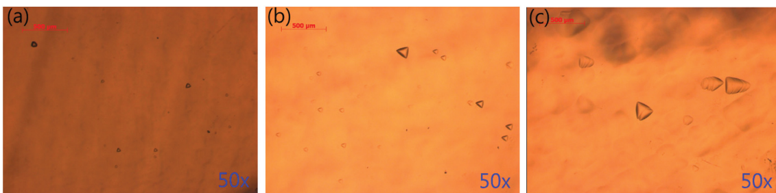
Fig. 3. OM images of Er(7.3%):YAG single crystal etched in H 3 PO 4 at 260°C for different times: (a) 20 min, (b) 1 hr, and (c) 1 hr 30 min.
