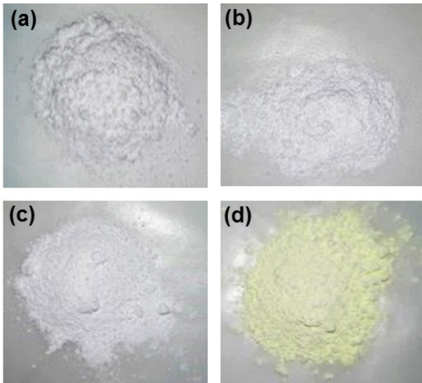
Fig. 3. Optical images of (a) MgO (b) \text{Al}_2\text{O}_3 , (c) \text{MgAl}_2\text{O}_4 , (d) \text{CeO}_2 ceramic pigments.
