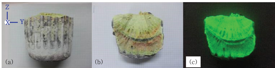
Fig. 2. Photograph of phosphorescent phosphor \text{SrAl}_2\text{O}_4 : \text{Eu}^{2+}, \text{Dy}^{3+} ingot; (a) before split and (b) cross section (c) under darkness of the synthetic ingot by skull melting method.
