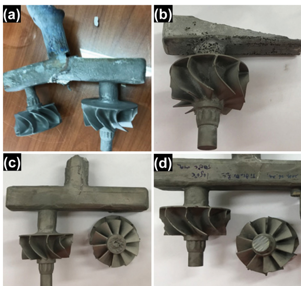
Fig. 2. Centrifugal casting results on the kinds of ceramic molds using (a) zirconia, (b) yttria, (c) alumina, and (d) alumina mixed with Ti powder.
