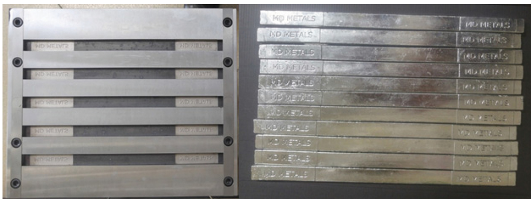
Fig. 1. Casting molder and Sn-3.0Ag-0.5Cu (wt%) solder bar sample.
