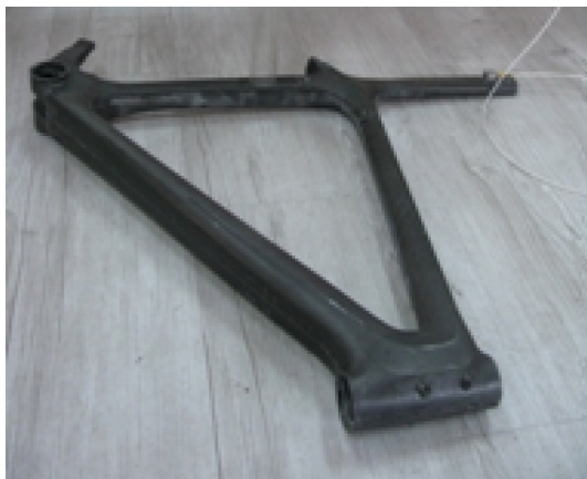
Fig. 8. Designed CFRP CNT frame.
