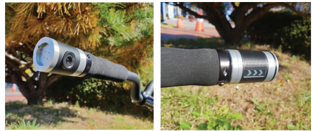
Fig. 15. The photographs of set to bicycle handle cam (a) and turn signal and speaker (b).
