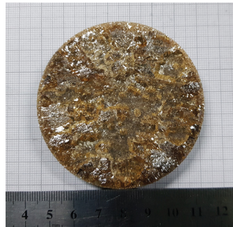
Fig. 2. A photograph of as grown crystal of AlN having a diameter of 3 inch for 120 hours in 1st growth.
