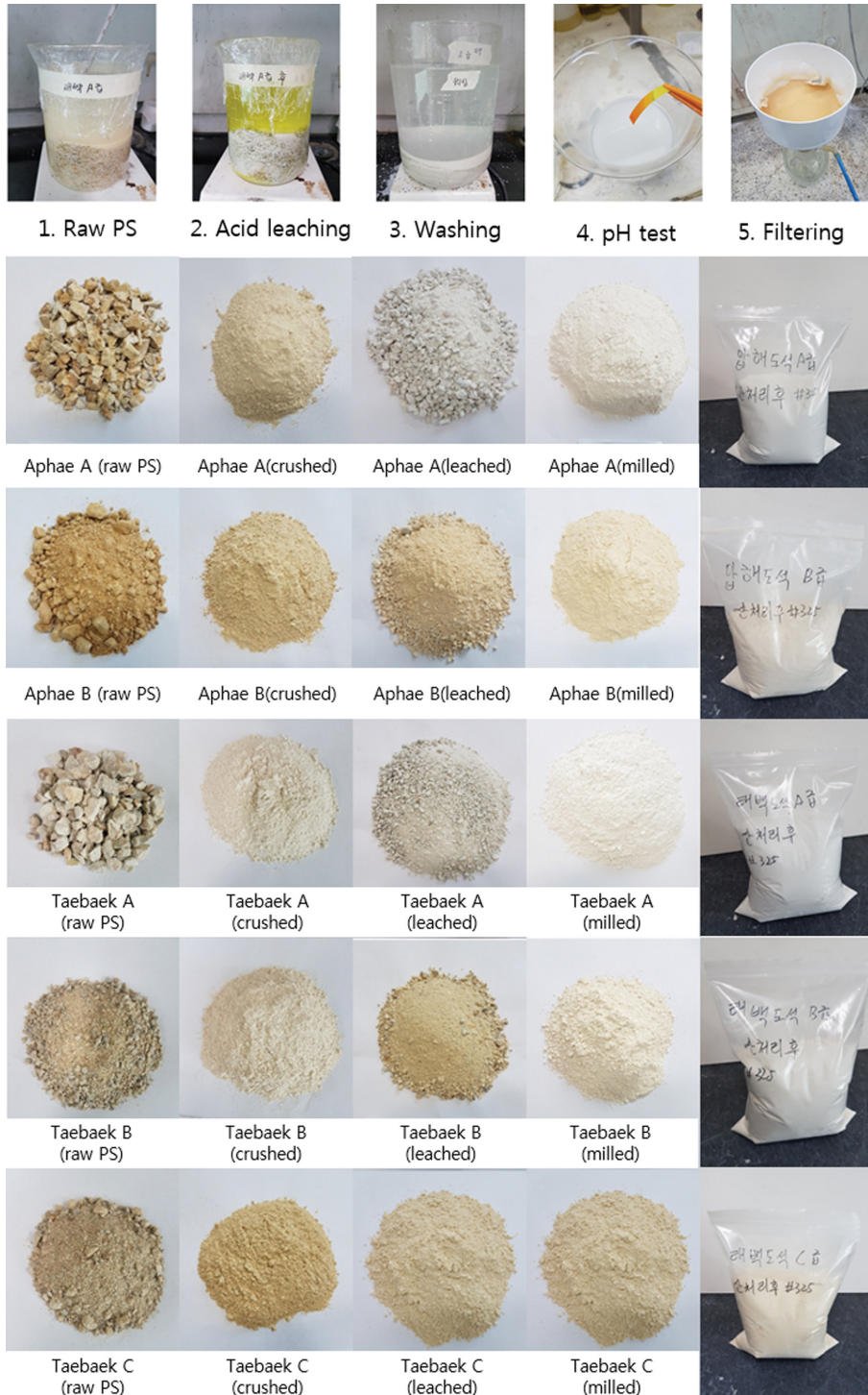
Fig. 1. Acid leaching process for refining pottery stone.
