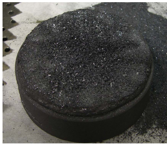
Fig. 6. Residue of SiC powder after crystal growth.
