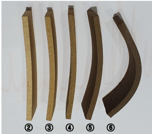
Fig. 4. Result of load testing of sample bodies sintering at 1,235°C.
