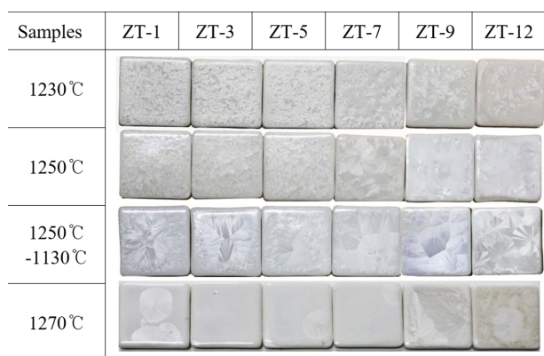
Fig. 5. Appearances of Zn_2TiO_4 additives as nucleating agent on willemite frit glaze by firing temp.
