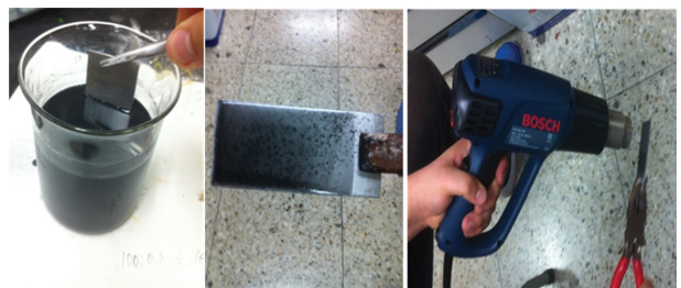
Fig. 1. Dip-coating and heat-treatment for the films requiring curing.
