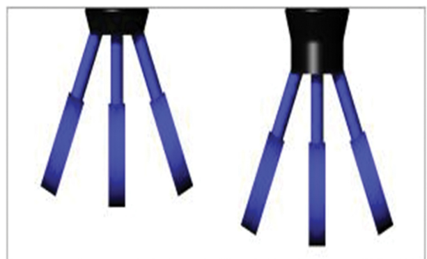
Fig. 3. Example of structure and angle of small sprue.
