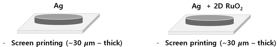
Fig. 3. Schematic diagram of the Ag current collectors coated on alumina substrate.
