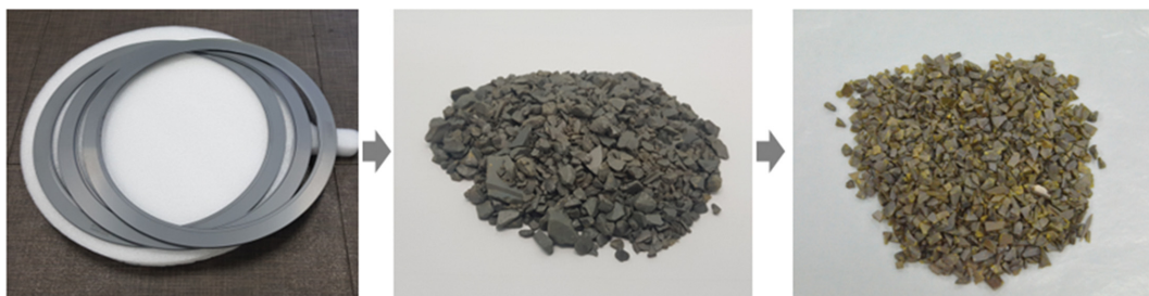
Fig. 1. SiC recycled powder: (a) focus ring, (b) granulated powder, (c) fine powder.
