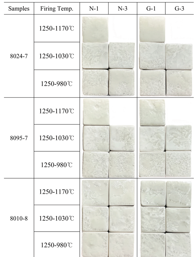
Fig. 11. Appearances of composition 8024-7, 8095-7 and 8010-8 with nepheline syenite as N, gerstley borate as G by annealing at 1170°C, 1030°C and 980°C.
