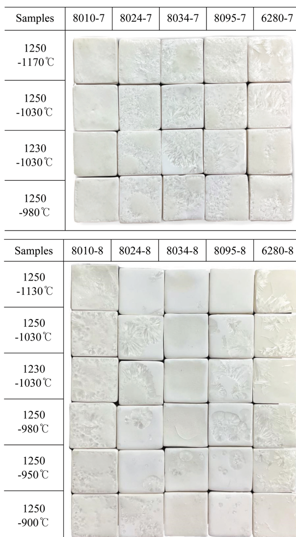
Fig. 6. Appearances of willemite glaze compositions 7and 8 of 8010, 8024, 8034, 8095 and 6280 by annealing temp.
