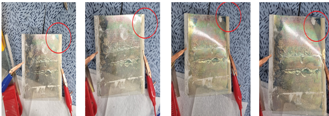
Fig. 6. Pictures of ECS film showing the color change from tinted state to transparent state under DC 3.5 V.
