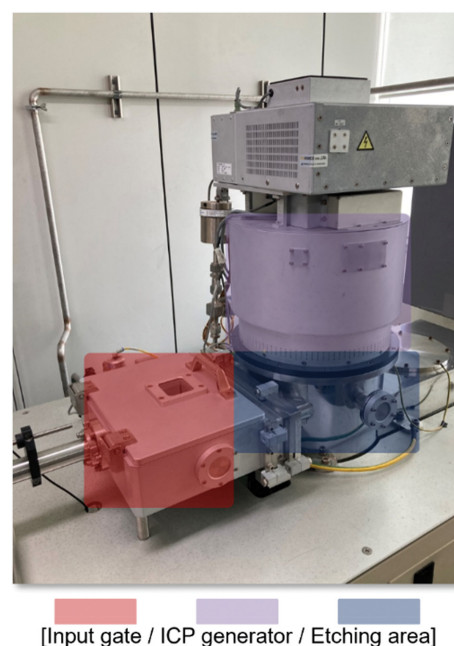
Fig. 2. External view of the ICP-Etcher, highlighting key functional areas: input gate (red), ICP generator (purple), and etching area (blue).
