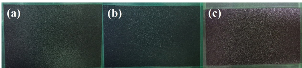
Fig. 10. Optical image after 72-hour salt spray test of PTFE-ZnO Primer: (a) PZ0, (b) PZ5, and (c) PZ5A.
