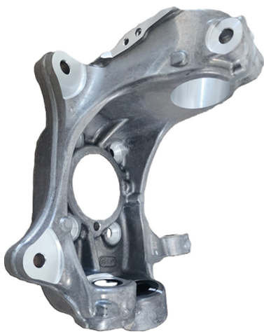
Fig. 1. Front Axle Knuckle (Hyundai Genuine OEM 51710AR500 Front Axle 4WD Knuckle LH for GENESIS GV70 EV 2022~2024).
