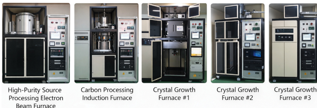
Fig. 2. Auxiliary material processing and growth furnaces for single crystal growth.
