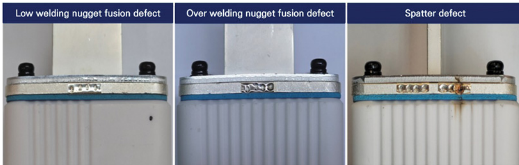
Fig. 5. Welding nugget defects of welding process by current manual work process.
