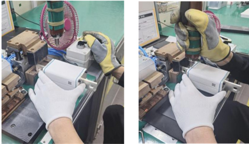
Fig. 4. Current spot welding process of BPU DC FUSE Elements by manual work.
