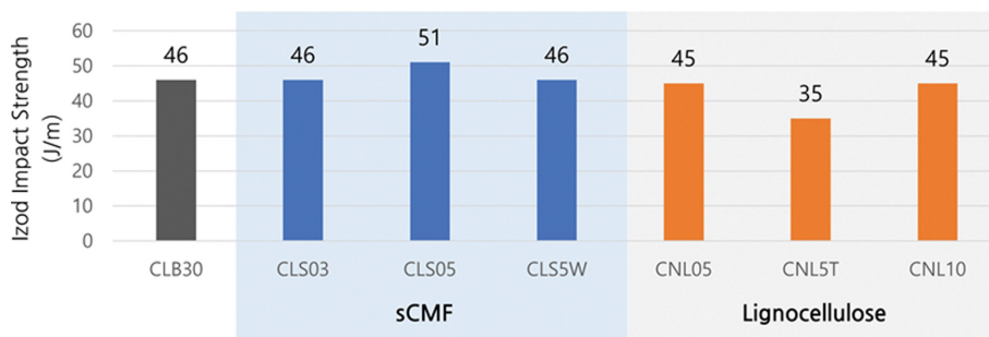
Fig. 4. Izod impact strength of PP composites containing sCMF and lignocellulose.
