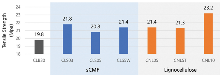
Fig. 3. Tensile strength of PP composites reinforced with sCMF and lignocellulose.
