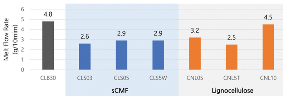
Fig. 5. Melt flow rate (MFR) of PP composites according to the type and content of modified cellulose-based fillers.
