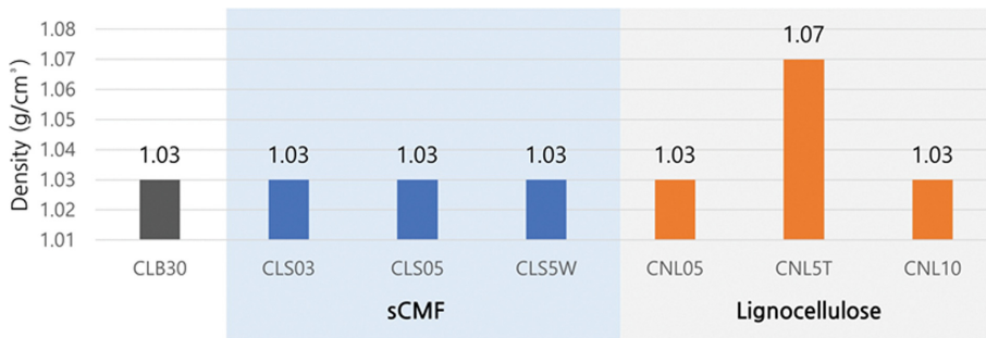
Fig. 2. Density values of PP composites containing sCMF and lignocellulose.
