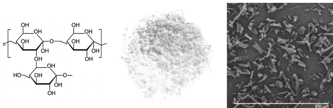
Fig. 2. Cellulose chain structure (left), cellulose powder (center), SEM image (right).
