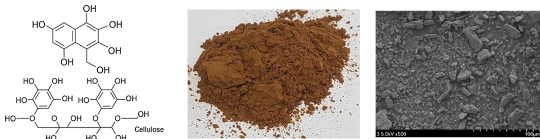
Fig. 3. Lignocellulose chain structure (left), lignocellulose powder (center), SEM image (right).
