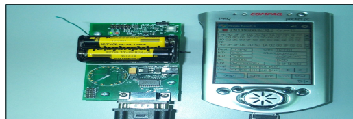
Fig. 6. Composition of Wireless Biosignal Acquisition System
