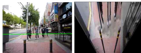
(a) Perspective-view image (b) Top-view image Fig. 3. An example of top-view transform.
