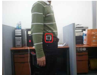
Fig. 14. Wearable devices mounted on the right of the belt.
