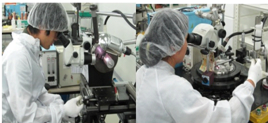
Fig. 3 Metal bellows welding operation by human being with microscope.
