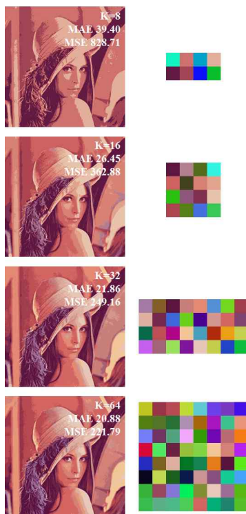
(a) Quantized Image (b) Used Palette Fig. 1. Results of K-means Color Quantization
