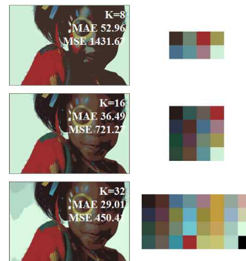
(a) Quantized Image (b) Used Palette Fig. 2. Results of Octree Color Quantization
