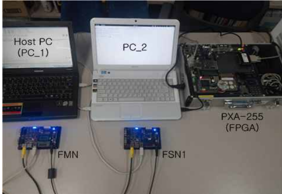
Fig. 12. The implementation environment for vehicle SoC fault diagnosis platform
