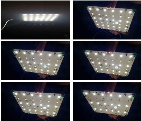
Fig. 14. Dimming Control by Visual Response
