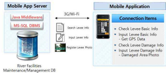
Fig. 2. Modules Diagram of the Levee Inspection System(Ministry of Land, Infrastructure and Transport)
