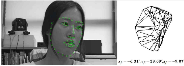
Fig. 7. Head pose estimation using POSIT
