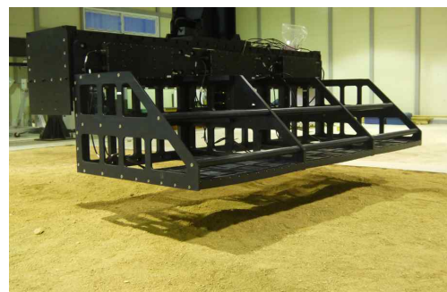
Fig. 5. MD performance test using the electrical controlled 3-axis scanner.
