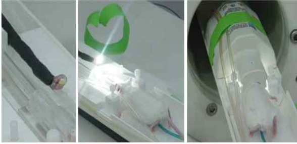
Fig. 1. Manufactured LED for light stimulation, and access on 9.4T MRI system
