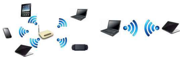
Fig. 3. Wi-Fi Infrastructure Mode and Ad-hoc Mode
