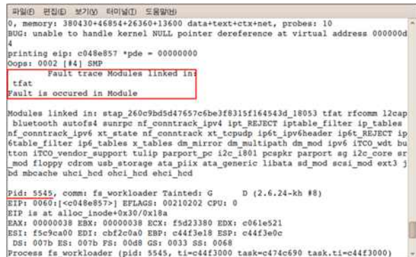
Fig. 7. Detection of Fault Generated by Fault Injector
