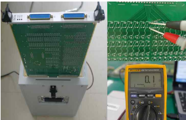
Fig. 9. Relay control test on VME expansion card
