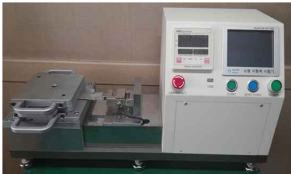
Fig. 6. Photo of manufactured separation force measuring system
