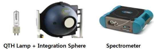
Fig. 2. Image acquisition equipment for radiometric Calibration
