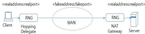
Fig. 2. Port and address hopping architecture
