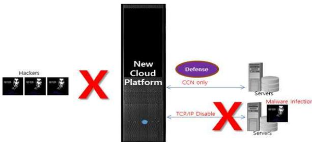
Fig. 11. Unable to communicate directly with TCP/IP in the internal network
