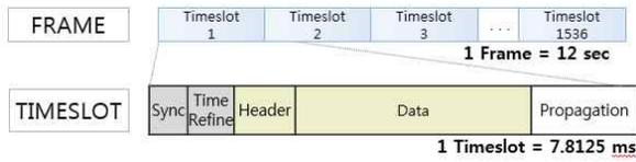
Fig. 1. TDMA Frame structure
