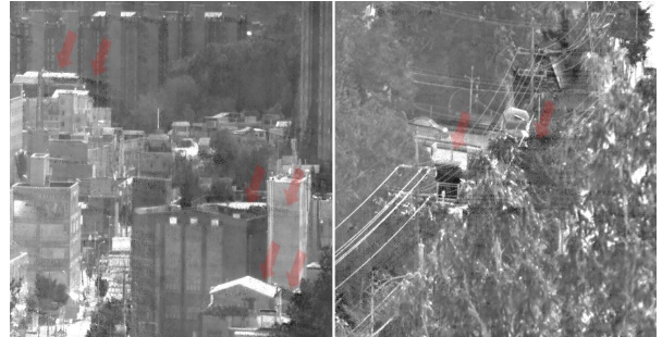
Fig. 8. Ghost effect (Due to large signal difference between average and ROI)
