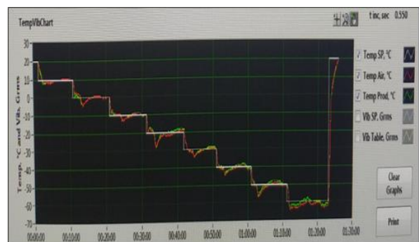
Fig. 7. Cold Step Test Result(Temperature)
